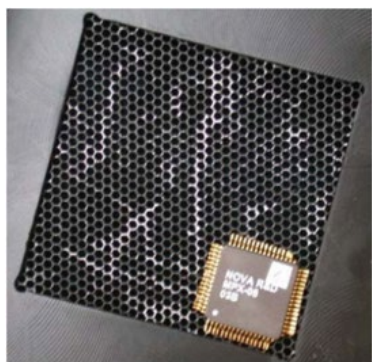
50 x 50 mm 2 collimator used in an experimental \gamma -camera (INFN former Scintirad Project);
