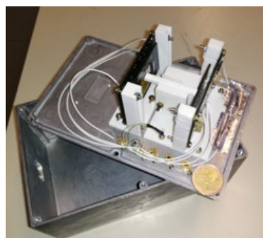
The ProtoXGS-2 prototype. A single 4.5 x 4.5 x 45 mm 3 scintillator bar is coupled at both ends with single cell, 5 x 5 cm 2 SDDs each with a PA-001 preamplifier.
