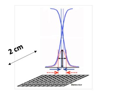
Produce highly segmented polycrystalline diamond dosimeter to obtain spatial distribution of small fields. Test to directly bond microwires over graphite pads to avoid the metalization step and have an all-carbon detector
