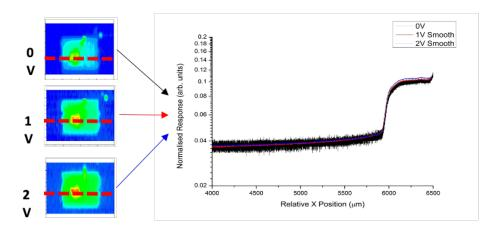
Surface scan of same sensors using microfocalized Synchrotron radiation at different biases.
