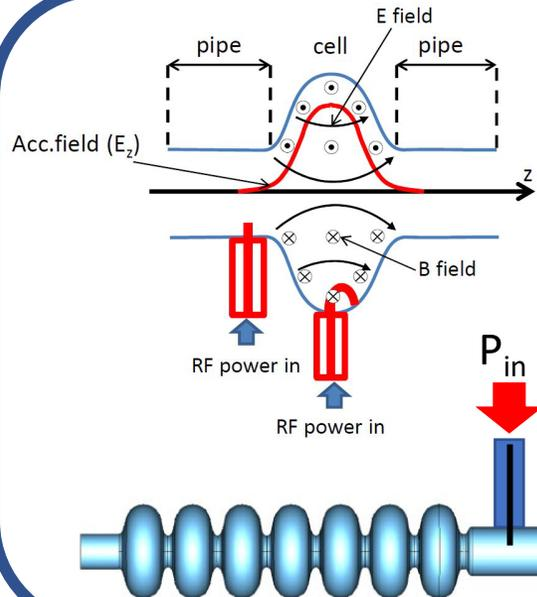
For a **pure cylindrical structure** (“pillbox cavity”) the first accelerating mode (i.e. with non-zero longitudinal electric field on axis) is the **TM<sub>010</sub> mode**. It has a well-known analytical solution from Maxwell equation. **Real cylindrical cavities: TM<sub>010</sub>-like mode** (because of the shape and presence of beam tubes).
