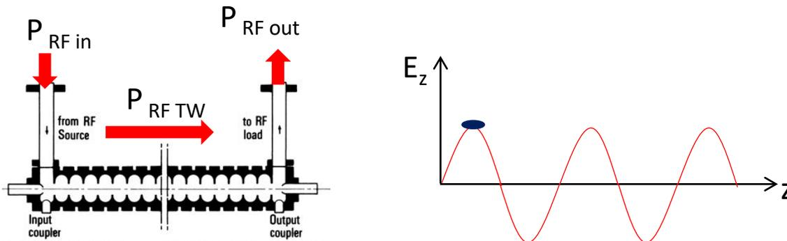
Typically, these structures are **used only for electrons** because  $v_{ph}$  can be assumed equal to  $c$  all along the structure.
