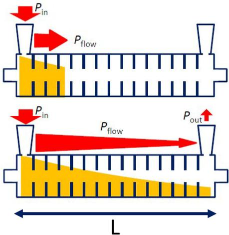
In a purely periodic structure, made by a sequence of **identical cells** (called “**constant impedance - CI**”), the RF power flux and the intensity of the accelerating field decay exponentially along the structure:
