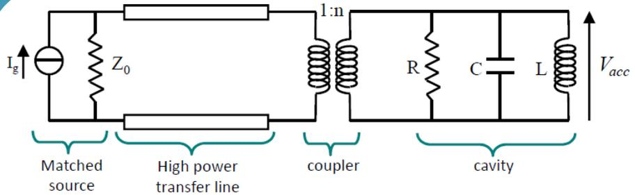
$$R = \frac{\hat{V}_{acc}^2}{P_{diss}} [\Omega] \quad Q = \omega_{RF} \frac{W}{P_{diss}}$$
