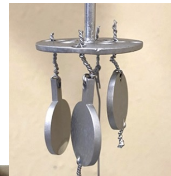
Nb 3 Sn target by dipping
