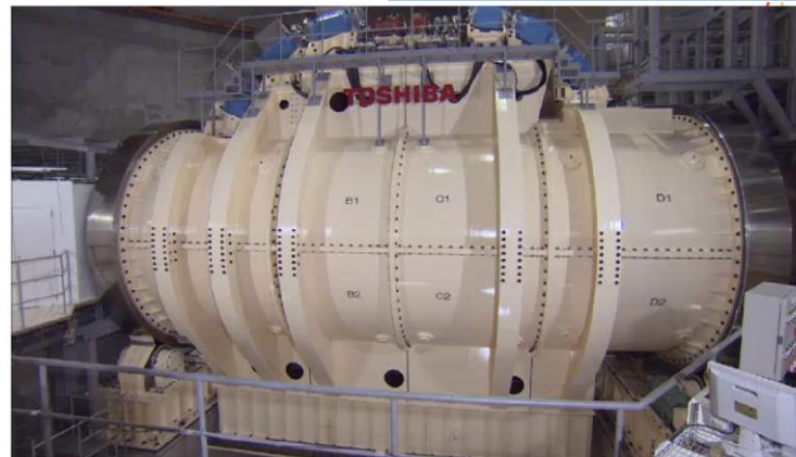
~300 tons, 11m diameter, 13m length
