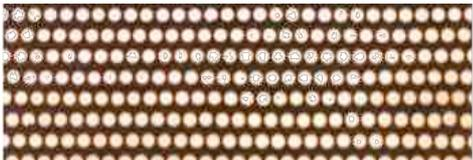
50 000 fibers,  $\phi = 1$  mm distributed uniformly inside 600 Kg of lead
