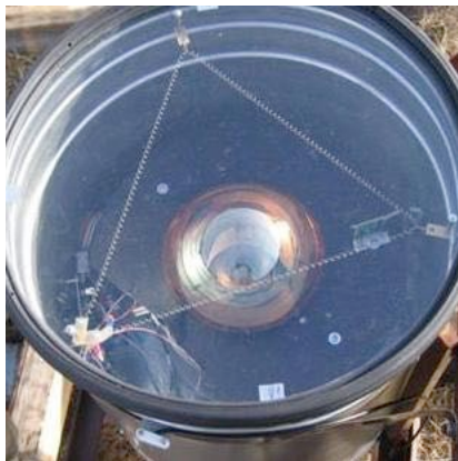
Tunka-133 - 175 optical detectors on the area 3 km 2
