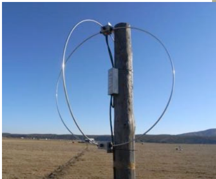
Тунка-REX – 45 antennas for registrations of radio signals From EAS
