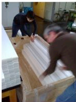
Extruded scintillator bars (1600 x 50 x 10 mm)
