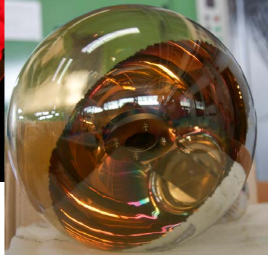
Novel MCP based devices from Chinese producer Transmission + reflective photocathode
