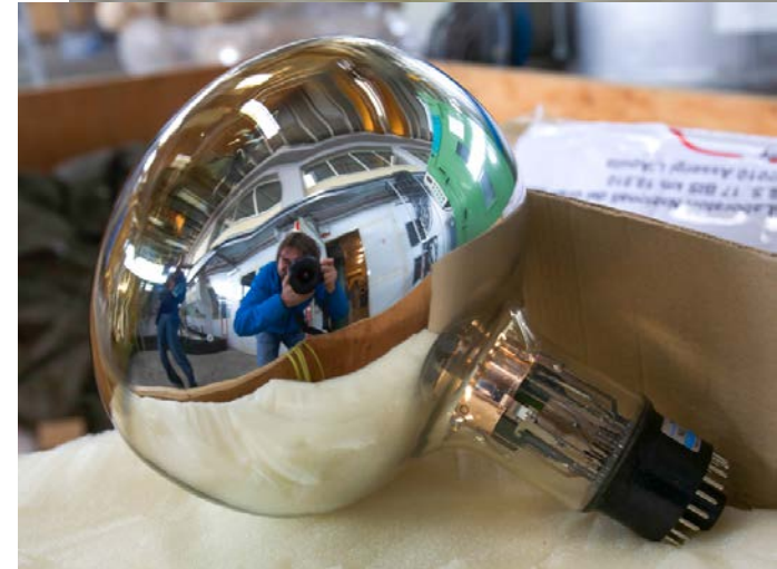
Novel MCP based devices from Chinese producer Transmission + reflective photocathode
