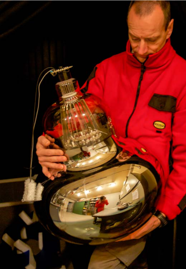
Hamamatsu 20 inches device evolved from the SK type Transmission photocathode
