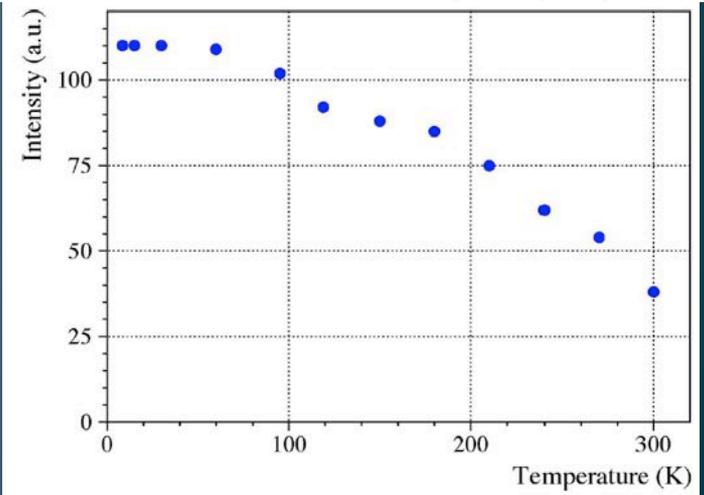
Light output measured for a ZnWO<sub>4</sub> scintillator<sub>9</sub> with <sup>241</sup>Am α particles as function of Temperature
