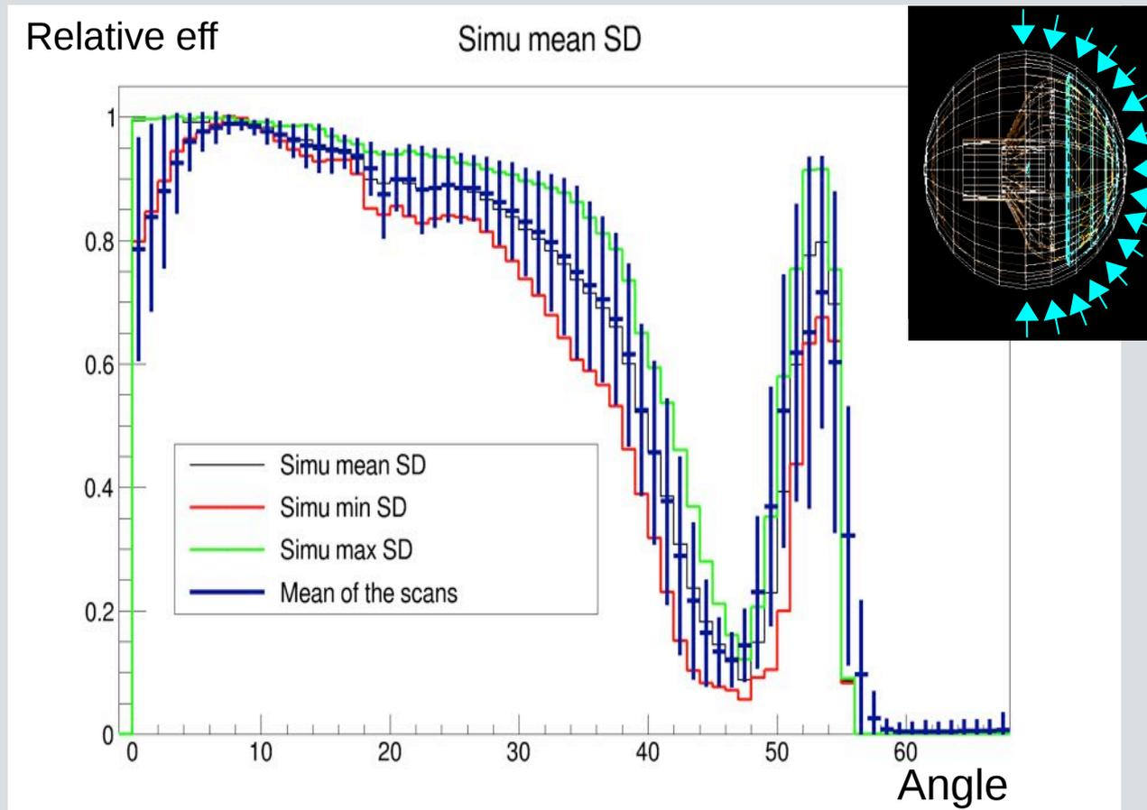
Very good fit between the simulation and data measurement done in laboratory on the different Optical modules
