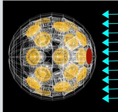
The angular acceptance corresponds to the probability that a beam of photons is detected by the optical module
