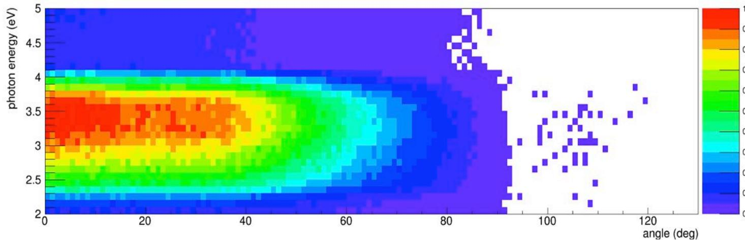
Angular efficiency in function of the angle and photon energy of one DOM PMt without reflector
