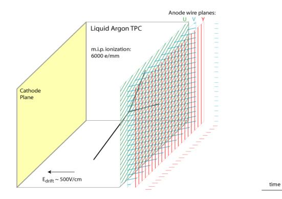
When a neutrino interacts with liquid argon it produces charged particles that deposit their energy, creating ionization electrons and scintillation light
