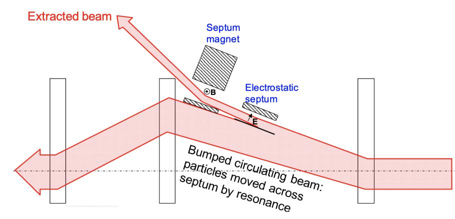
A fraction of the particle beam interact with the matter in the septum and generates losses
