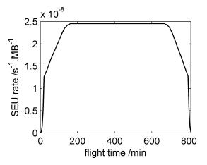
Neutron flux increases as rigidity cut-off decreases (at high latitudes). Expect c. 1 event per gigabit per transatlantic flight.
