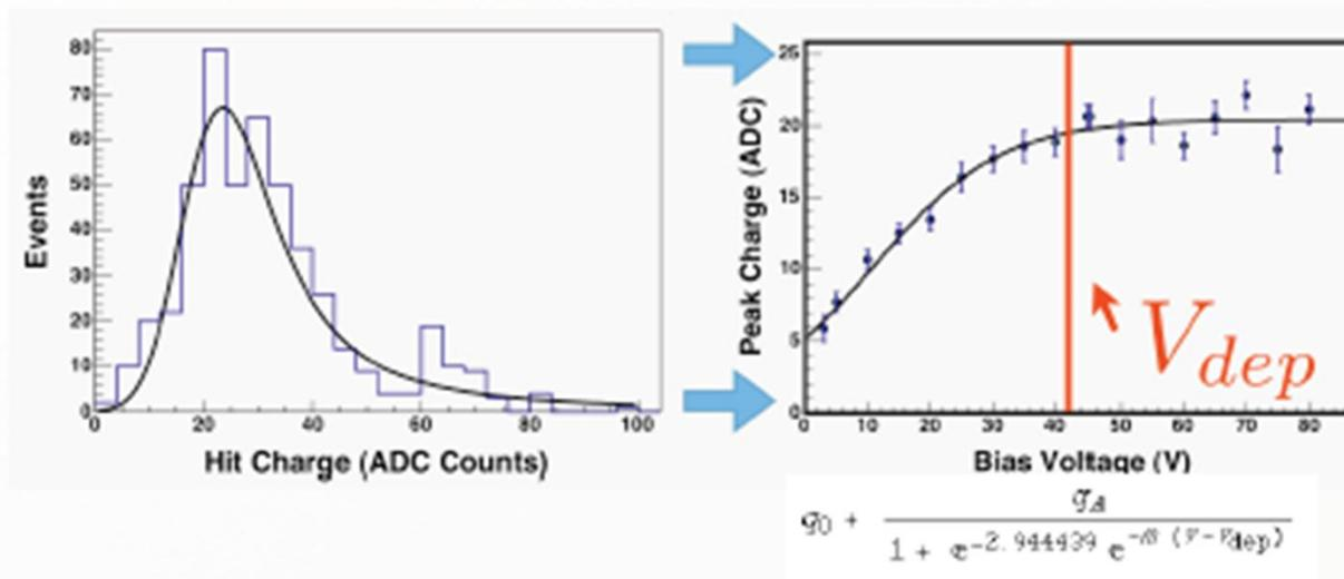
Fit signal charge (hits on tracks) to Landau  $\otimes$  Gaussian
