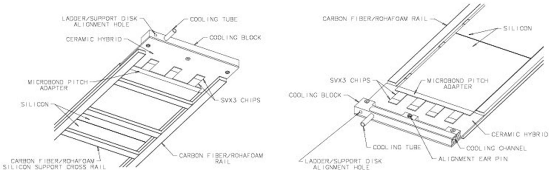
Figure 6.4: A close up view of the readout hybrid on the stereo side of a ladder (left) and the readout hybrid and cooling channel on the axial side of a ladder (right).
