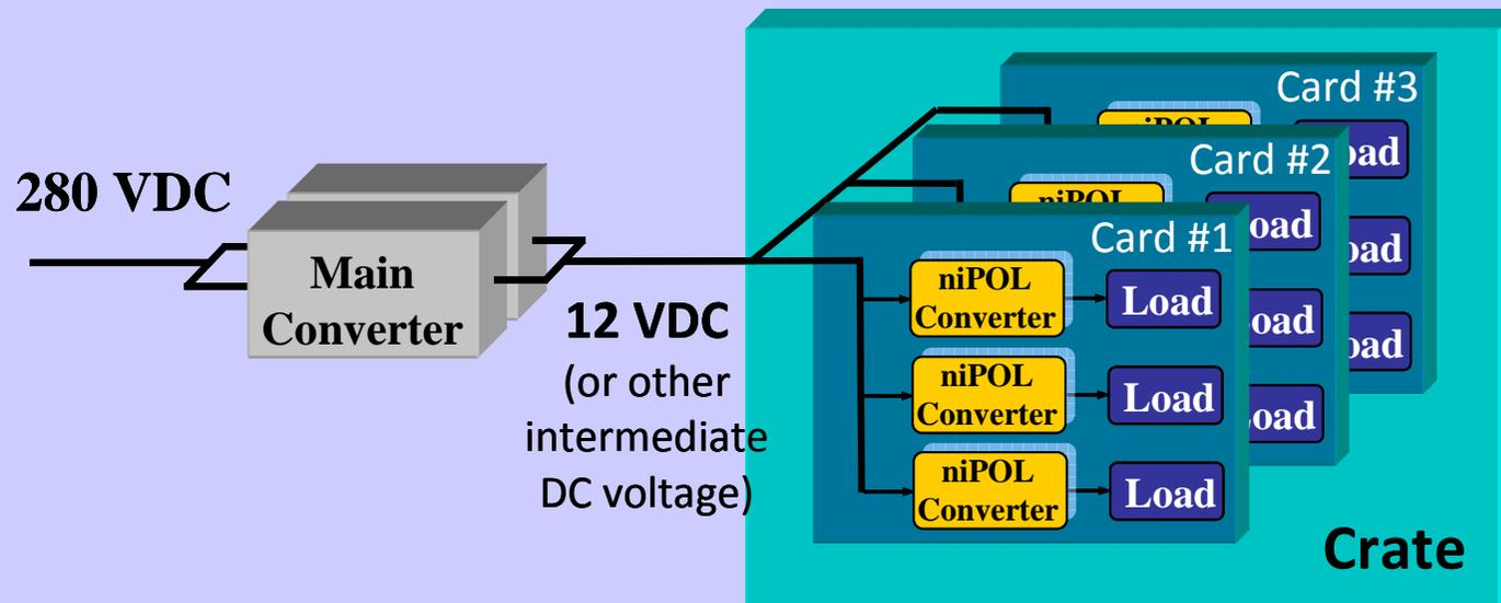
niPOL = Non-Isolated Point of Load Converters
