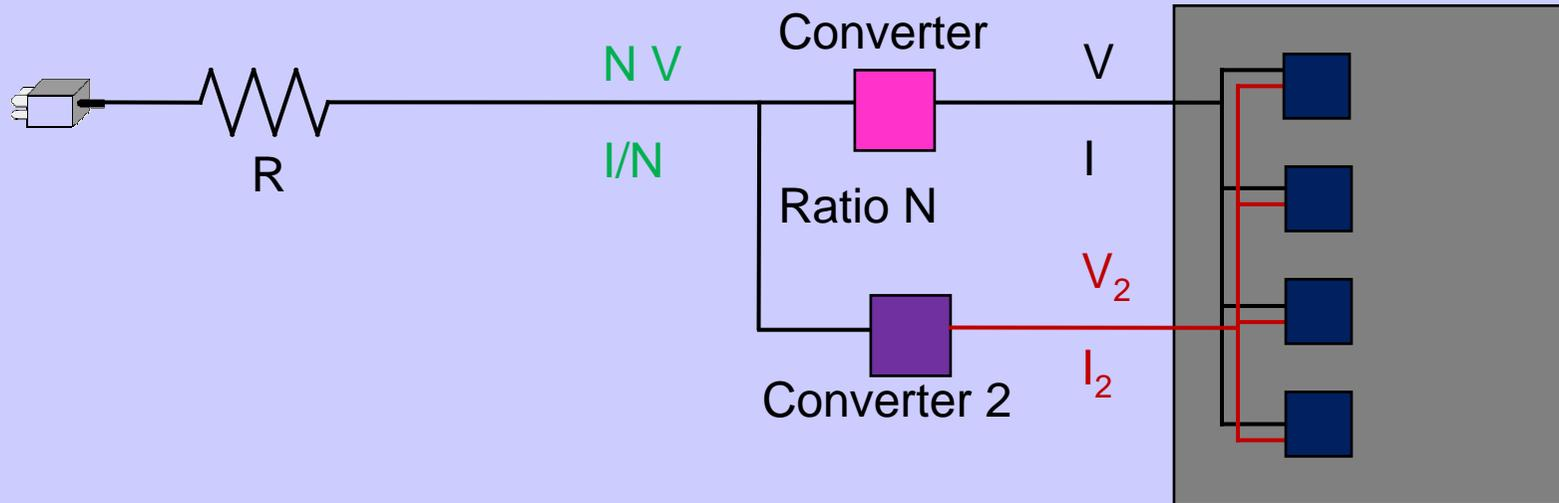
Solution without converter: ↓ Power losses on cable =  $RI^2$
