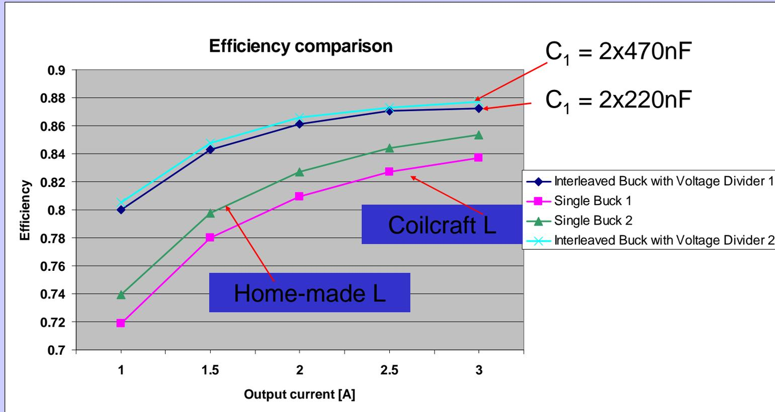
*Home-made L*: 0.84mm wire diameter ( $L = 220\text{nH}$ ,  $50\text{m}\Omega$ ) wound on a plastic support ( $\phi = 4.38\text{mm}$ )
