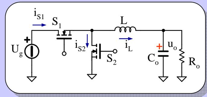
The 2<sup>o</sup> order  $L-C_o$  filter removes the switching frequency harmonics, making the output voltage DC component dominant
