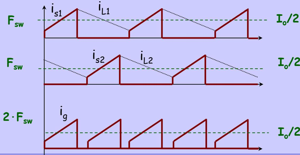
Ripple reduction on input current
