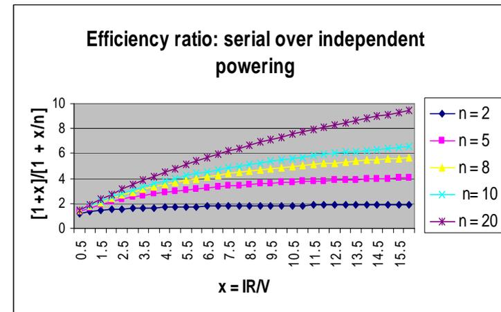
**Example of efficiency plot vs. number of modules (n) and supply voltage (V) for  $I_m = 2 \text{ A}$   $R_c = 3 \Omega$  for Serial Powering scheme**
