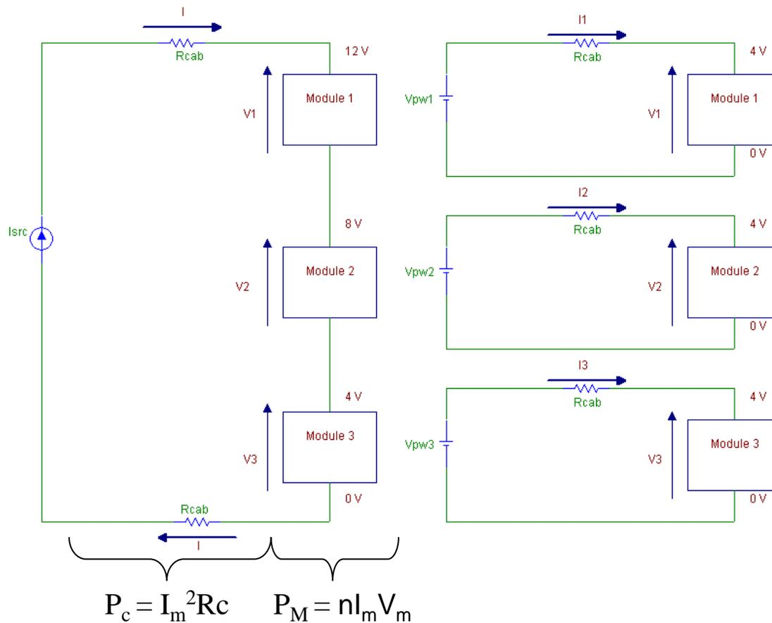
$$\text{Efficiency} := \eta := \frac{P_M}{P_M + P_C} = \frac{1}{1 + \frac{I_m R_c}{n V_m}} = \frac{1}{1 + \frac{x}{n}}$$
