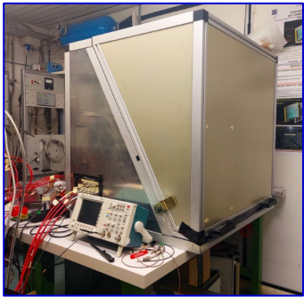
Initial dark-box; then, optimized dark-box modified to improve light-tightness and operative needs
