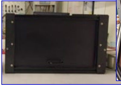
Initial dark-box; then, optimized dark-box modified to improve light-tightness and operative needs
