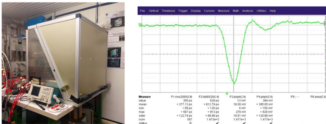
Fig. 6 The dark-box realized in TS to house the LAPPD (left) and the signal shape output from the LAPPD using an Agilent 33220A (right). A time time resolution of 35 ps was preliminary estimated.
