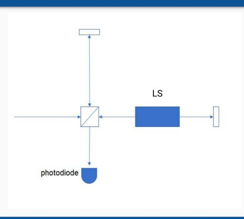
$v_a$ : Arrival time measurement Testing with several wavelengths Cuvette in one arm of interferometer with/without LS Interference fringes displacement V
