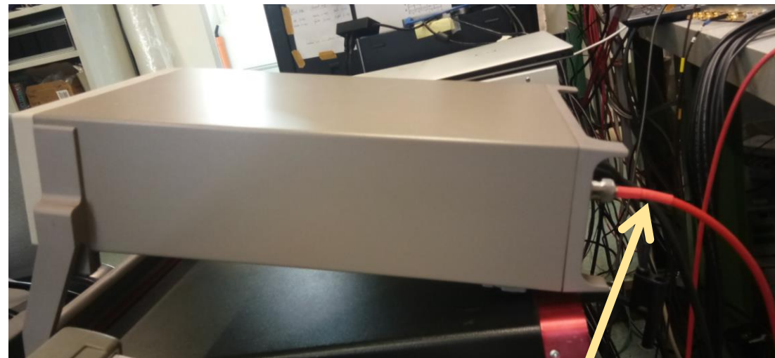
Lemo (via the HV cable) is terminated on Keithley input
