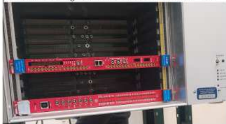
WEINER VME crate: CAEN V1718 controller board CAEN V1742 Digitizer board with 32 readout channels
