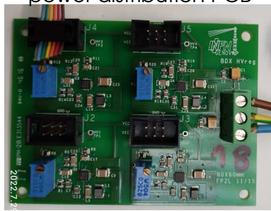
power distribution PCB
