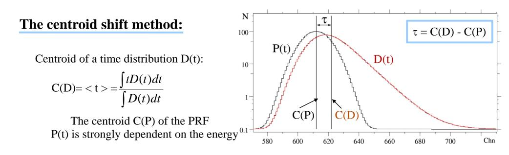
"The prompt curve" indicating  $\tau = 0$  is needed ! Example only one plastic scintillator. (time-walk characteristics)
