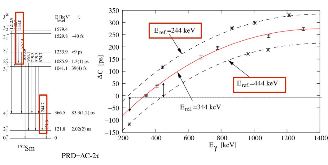
As the combined  $\gamma$ - $\gamma$  time-walk characteristics, the PRD curve is shifted in parallel using different reference energies (reference timing signals).
