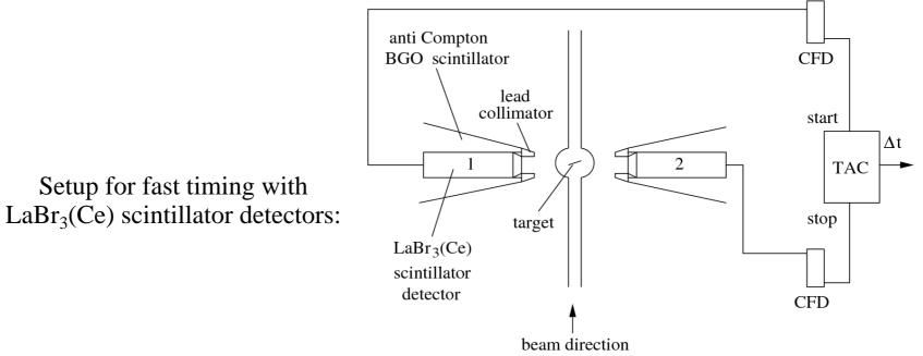
In-beam  $\gamma$ -ray spectroscopy with LaBr<sub>3</sub>(Ce) scintillator detectors
