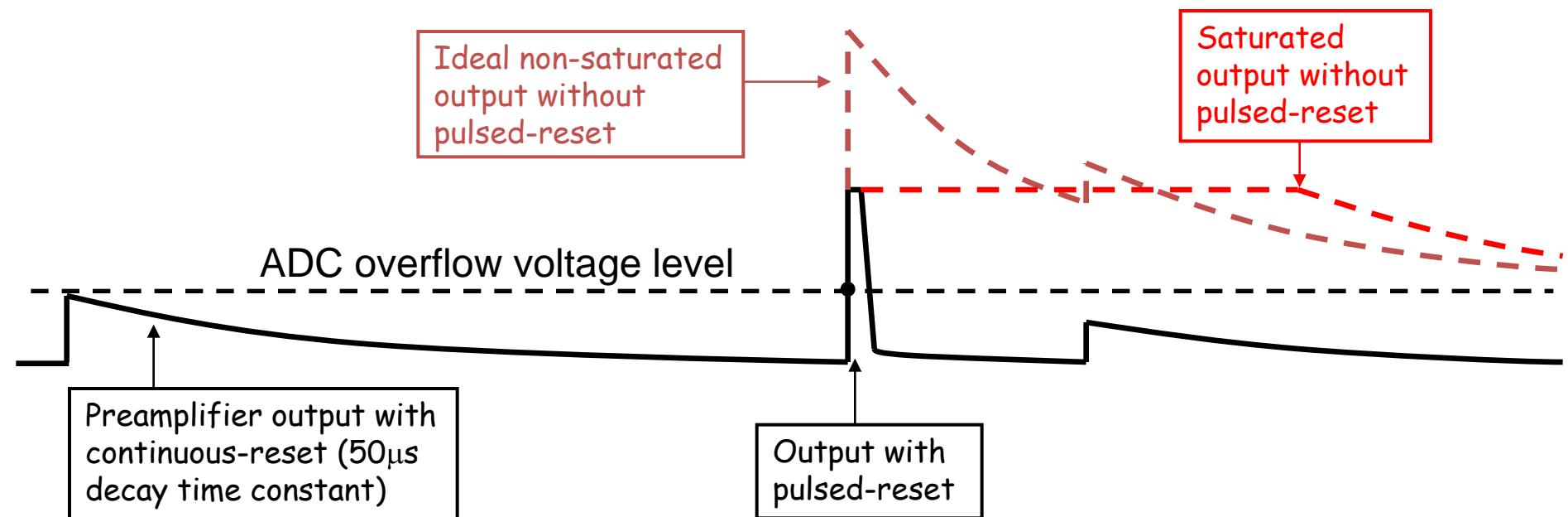
An ADC overflow condition would **saturate** the system for a long while
