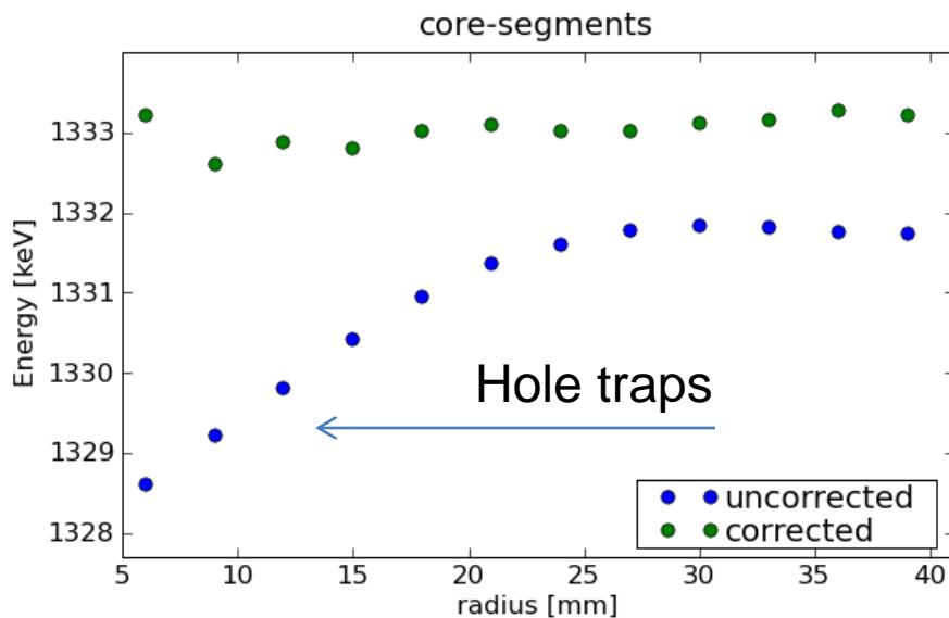
Neutron damaged detector:
