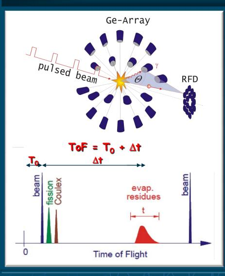
RFD is a HI detector that measures evaporation residues in coincidence with γ-rays detected in a Ge array
