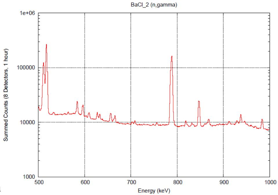
γ-ray spectrum of the energy range 500-1000 keV for a one hour in-beam measurement of a BaCl<sub>2</sub> target at PF1B
