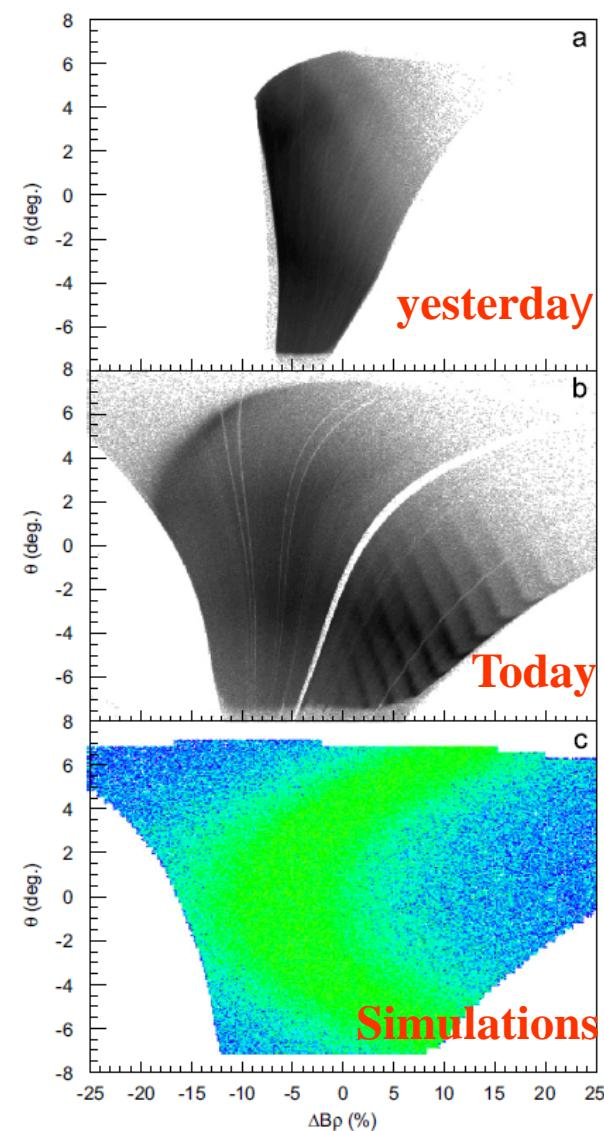
**Fig. 11.** Two-dimensional plot of  $\theta$  as a function of relative rigidity for transmitted trajectories. (a) Same as in Fig. 2(b) for a detector size of 400 mm  $\times$  110 mm. (b) From the present measurement with a detector size of 1000 mm  $\times$  150 mm. (c) Simulation for an isotropic distribution of particles entering the spectrometer, for a detector size of 1000 mm  $\times$  150 mm.
