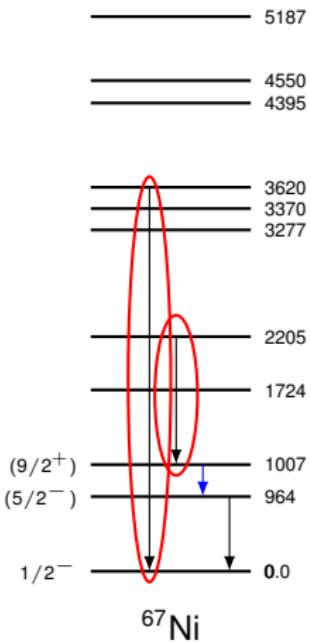
Indications of a populated level around 2.5 MeV which does not decay directly to the ground state  $\Rightarrow$  good candidate for  $\nu 2d_{5/2}$ -state ( $N=50$ )
