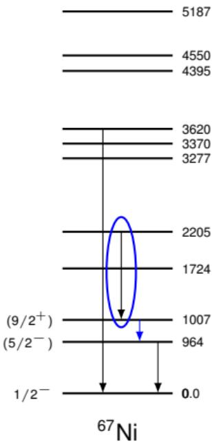
Indications of a populated level around 2.5 MeV which does not decay directly to the ground state  $\Rightarrow$  good candidate for  $\nu 2d_{5/2}$ -state ( $N=50$ )
