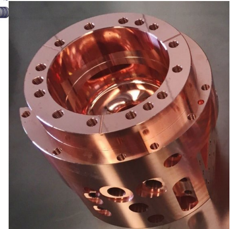
Body of the gun (single piece of OFHC copper)
