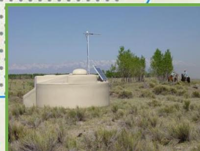
1665 surface detectors: water-Cherenkov tanks (grid of 1.5 km, 3000 km<sup>2</sup>)
