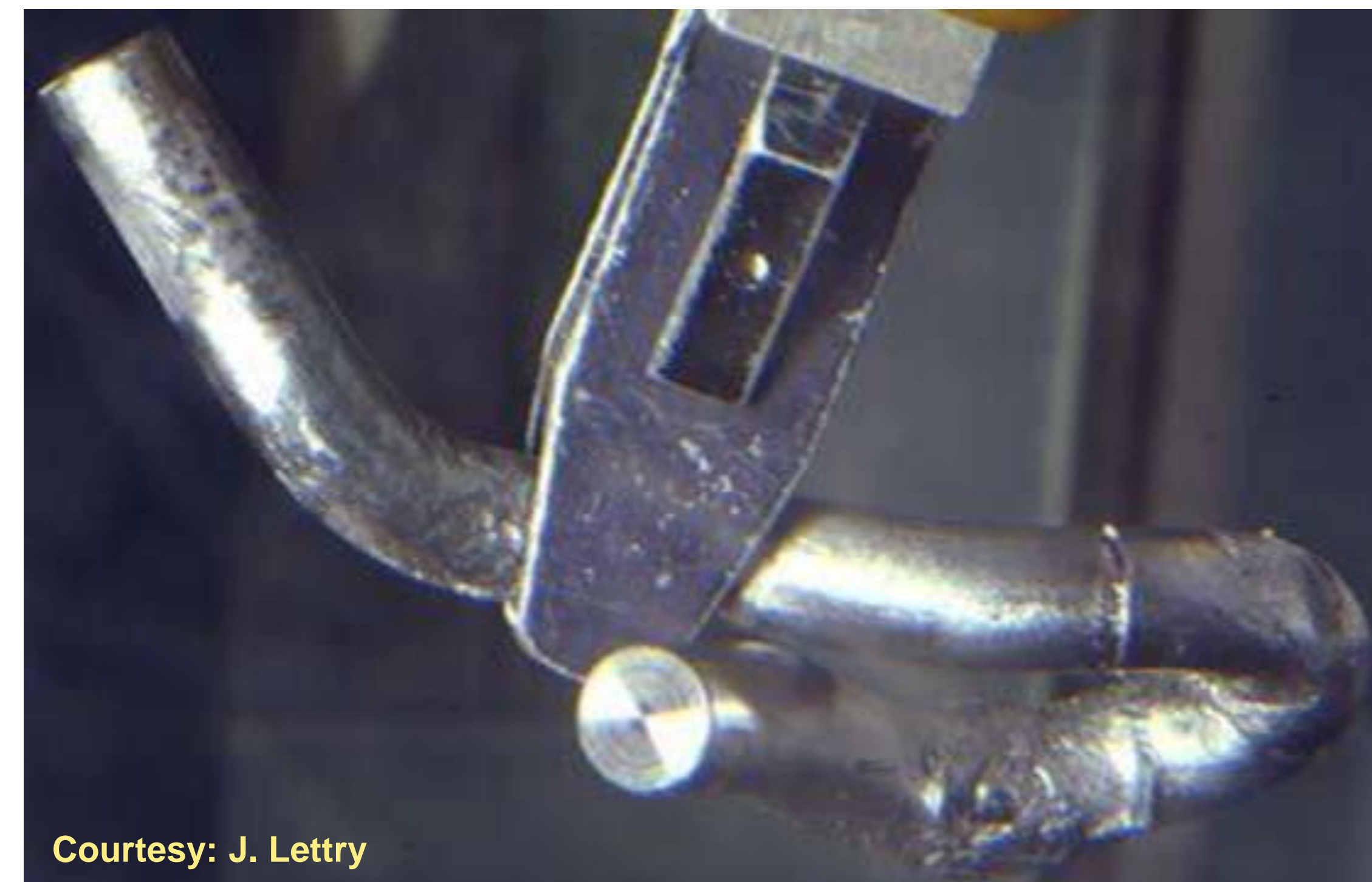
Ta rod after irradiation with 6E18 protons in 2.4us pulses @ 1.4 GeV/c (ISOLDE)
