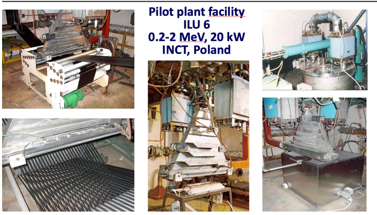
RAPID @ INCT Facility providing electron beams (0.2-10MeV, 0.1-20kW) and gamma irradiations (Co60) – 10MeV ns e-pulse for Radiolysis
