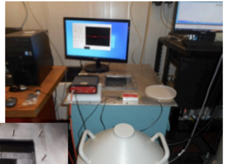
BEGe shielding opened (left), improved BEGe setup (right)
