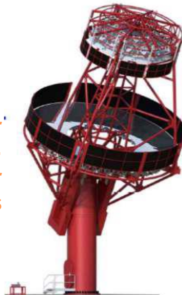
MST Dual Mirror Schwarzschild- Couder \sim 12k SiPMs
