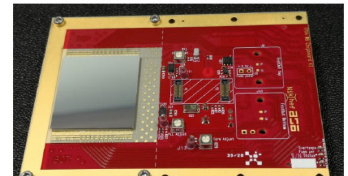
Timepix4v1 with full (512 x 448) Si sensor (March 2021)
