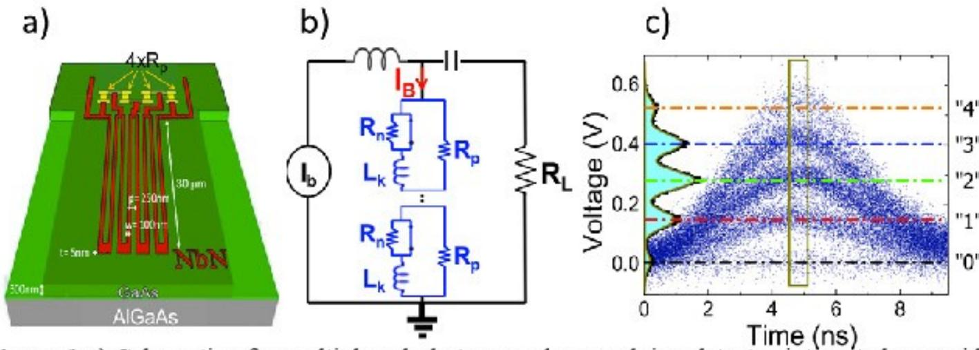
**Figure 1** a) Schematic of a multiplexed photon number resolving detector integrated on a ridge GaAs waveguide, developed using a series connection of four pixel SNSPD and b) its equivalent electric circuit, which includes the amplifier input impedance  $R_L$ . c) Pulse height corresponding to the number of absorbed photons [25].
