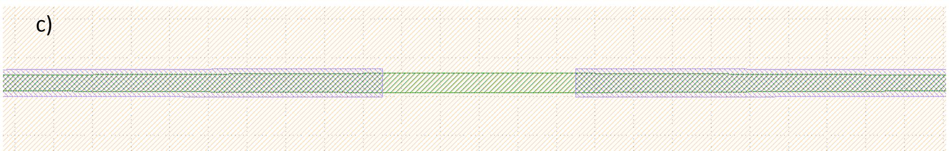
Nano device architectures for 2D-material-based polarization processor. The nanomaterial (graphene) lies onto the Si waveguide and is coupled to it a) Schematic view, b) Perspective view from Lumerical FDTD solver, c) Zoom in view from GDSII file of the chip with the exposed region for contacting with graphene of  $5 \times 50 \mu\text{m}$ .
