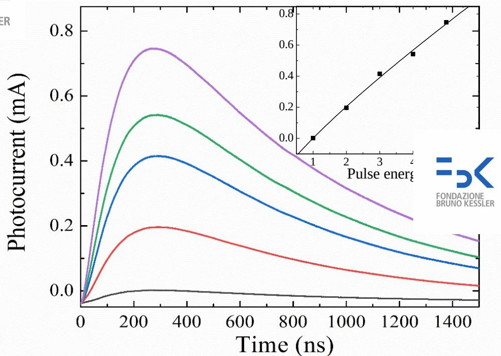
$\text{Bi}_2\text{Se}_3$ /n-Si response to fs laser pulse.
