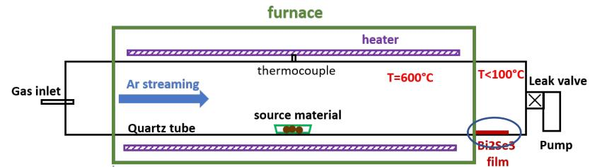
VSD furnace showing the quartz tube with source material and substrates
