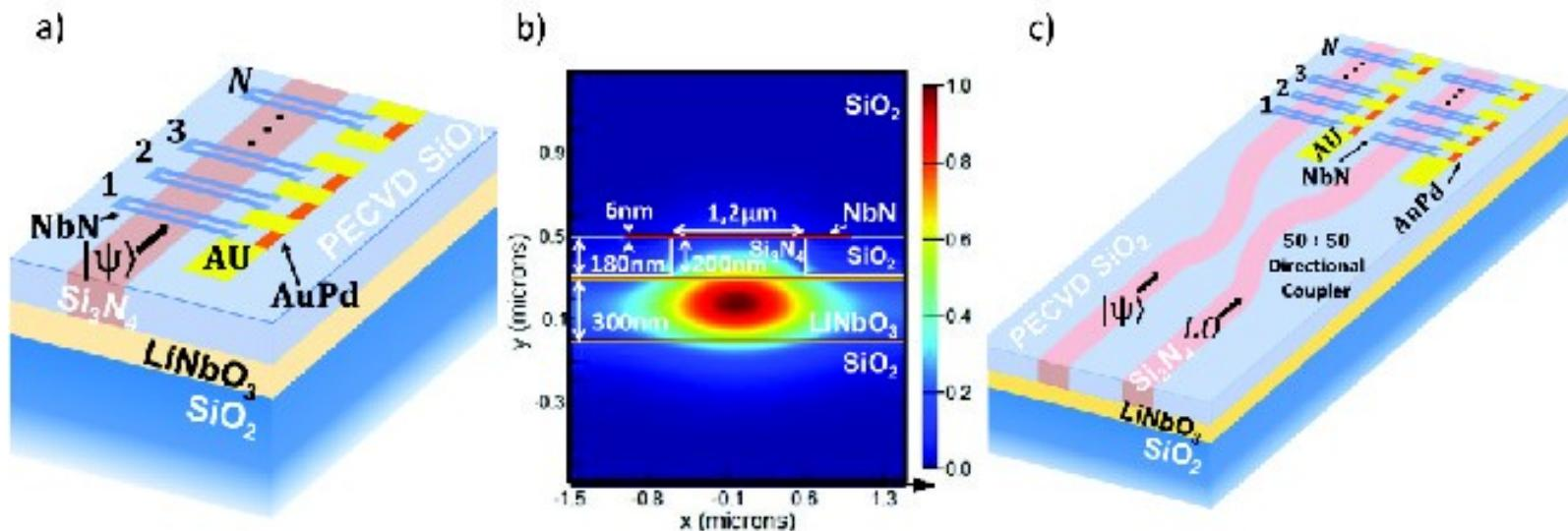
**Figure 2** a) Schematic of the integrated PNR to develop in this project showing a series of  $N$  pixels composed by a NbN nanowire (80 nm width) and an AuPd on-chip parallel resistance ( $R_p=20 \Omega$  value). b) Field intensity for the first TE mode propagating in the waveguide where the light absorption in each NbN nanowire element is at 3.4%. c) Schematic of the hybrid detector.
