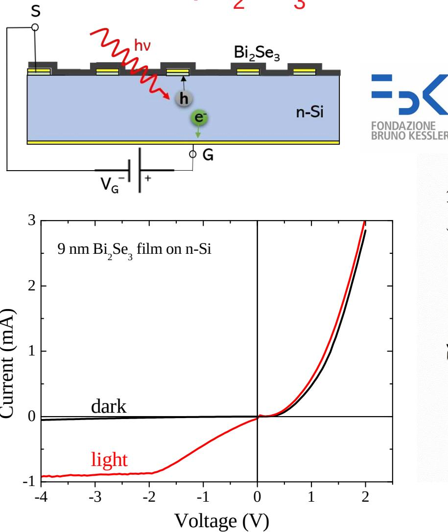
I-V characteristics of  $\text{Bi}_2\text{Se}_3$ /n-Si heterojunctions in dark and illuminated conditions (9 nm film).
