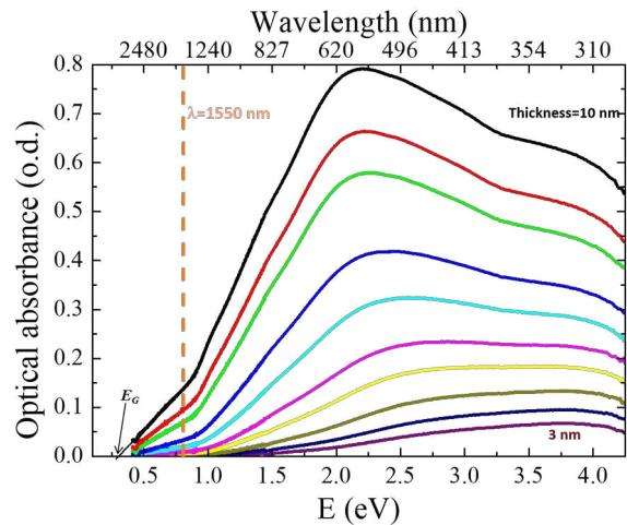
Optical absorbance at different energies with different film thickness
