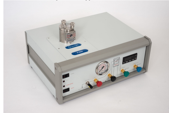
K850 critical point dryer (CPD) from Quorum
