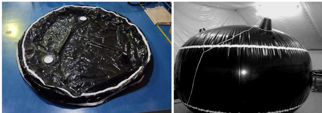
Figure 2.4: A liner from Auger observatory. Left: folded liner. Right: inflated liner for tests.
