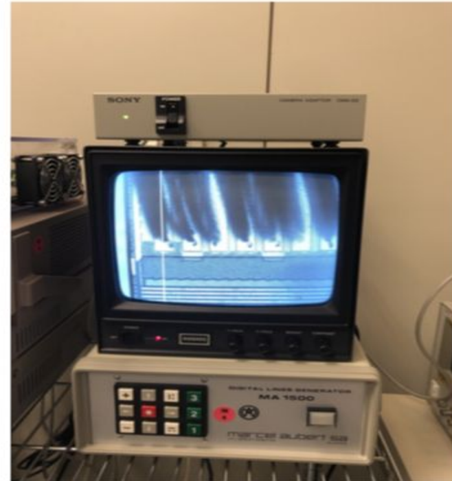
Probe-card alignment on MaPSA pads
