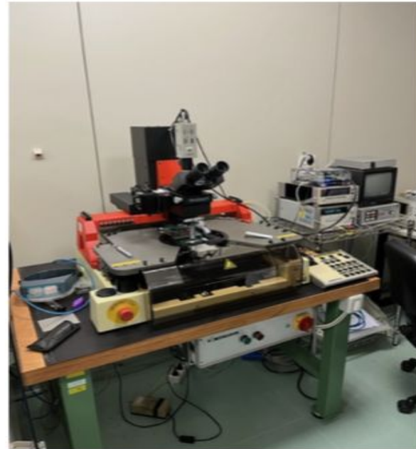
8" probe station setup in Padova for MaPSA testing
