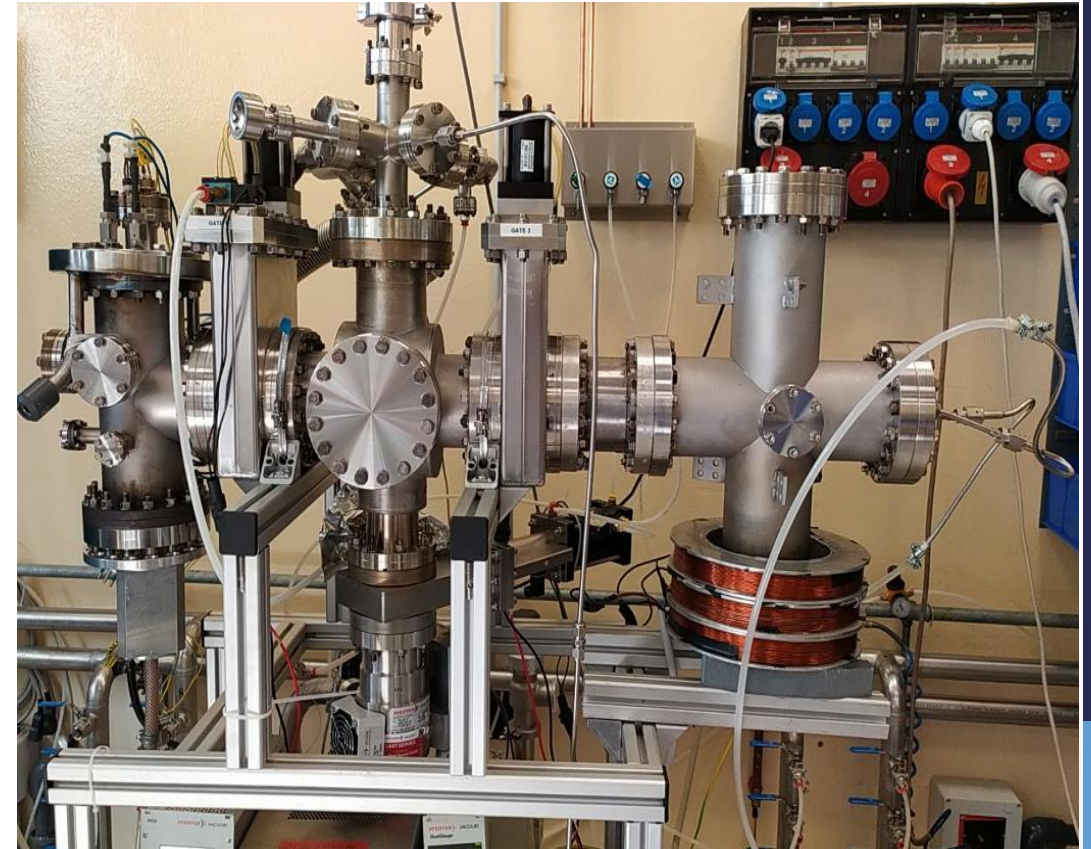
The vacuum system dedicated for inverted magnetron deposition test and future target production
