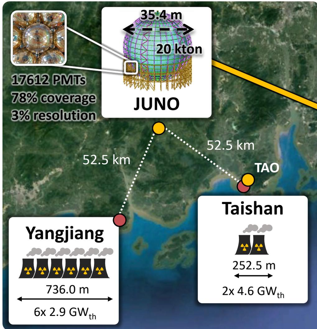
**JUNO** is a **20 kton** multi-purpose underground **liquid scintillator** detector currently under construction at a baseline of about **52.5 km** from eight **nuclear reactors** in the Guangdong Province of South China.
