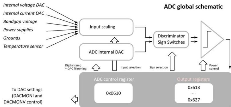
ALPIDE application-specific integrated circuit includes a **monitoring ADC** to measure quasi-static voltages and currents generated on chip, that also features a **temperature sensor**.
