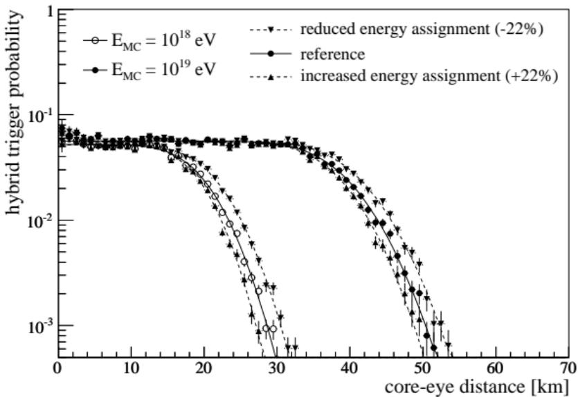
Trigger threshold dependence on a possible systematic energy shift removed by requiring the core to lie within a distance from the FD:
