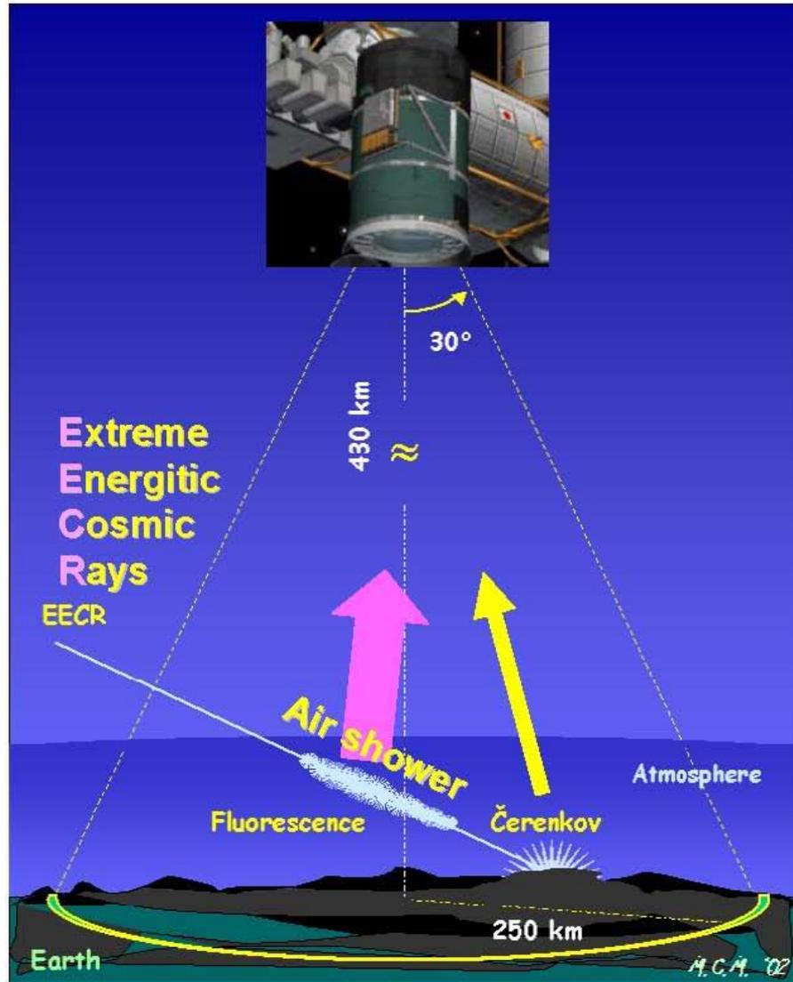
**JEM-EUSO is a new type of observatory on board the International Space Station (ISS), which observes transient luminous phenomena occurring in the earth's atmosphere.**
