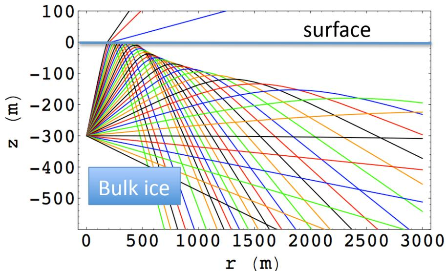
Shown: pathways for propagating radio waves emitted from a point at 300 m depth in ice.
