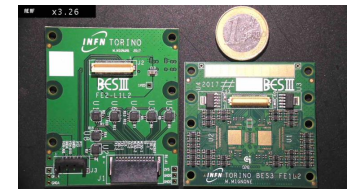
Front end board (FEB)
