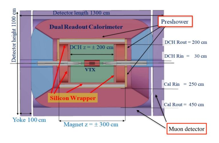
Preshower and the muon detection system are designed with the µRWELL technology
