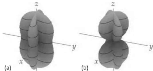
**Figure A.1** The beam pattern functions  $F_+^2(\theta, \phi, \psi = 0)$  (a) and  $F_\times^2(\theta, \phi, \psi = 0)$  (b) for an interferometric gravitational-wave detector with orthogonal arms along the x- and y-axes.
