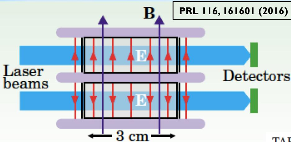
**Tabletop experiment at U. Washington (Seattle).** Laser beamed through two cells with Hg vapor. **Analysis phase**, light plane polarized  $\rightarrow$  nuclear **spin precessed around B**.
