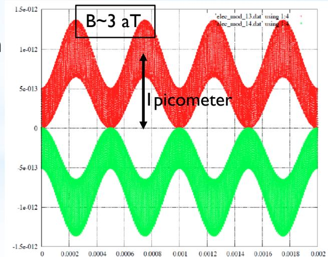
Figure 11.3: Simulation results for counter-rotating particles. The vertical beam position in meters [m] is shown here vs. time [s] for a constant radial B-field of 0.3 pG, and using eq. (11.7) to modulate the vertical tune (using  $f=1\text{KHz}$ ). The two colors correspond to clockwise (red) and counter-clockwise (green) rotations for an average radial B-field directed outwards in the radial direction.
