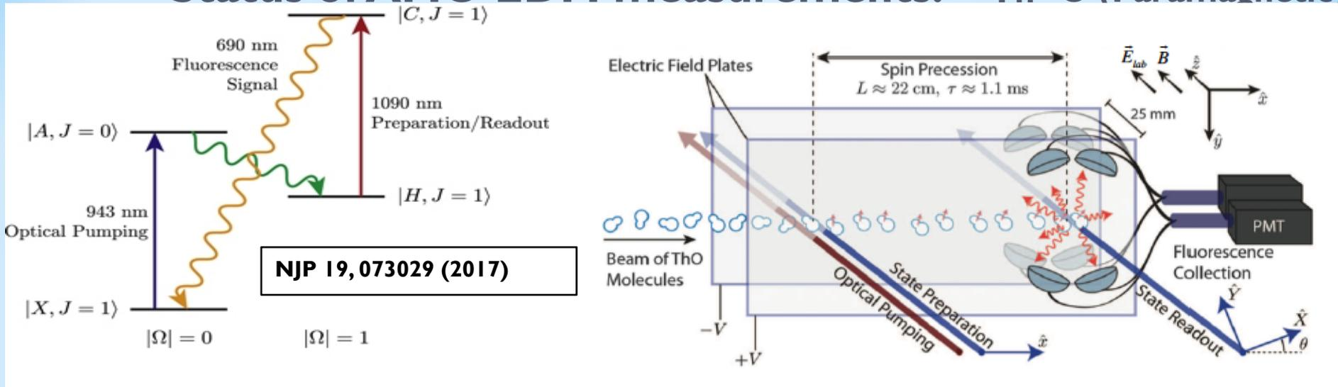
In **paramagnetic** systems with one (or more) unpaired  $e^-$ , EDMs are dominated by  $\mathbf{d}_e$  and the nuclear **spin-independent e-N interaction ( $\mathbf{C}_S$ )**. Great advantage is **large internal E-field (GV/cm)**.
