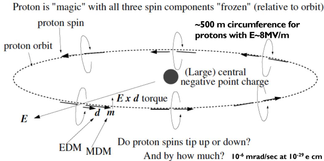
$$\vec{\omega}_a = -\frac{q}{m} \left[ a_\mu \vec{B} + \left( -a_\mu + \frac{1}{\gamma^2 - 1} \right) \vec{\beta} \times \frac{\vec{E}}{c} \right].$$
