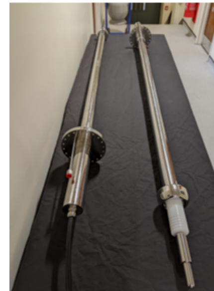
HV feedthrough completed (with spare)
