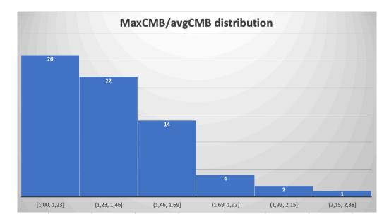
Typical distribution, over a quadrant (69 CMBs), of the Max-rate/AVG-rate ratio on a chamber
