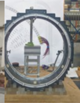
Carbon Fiber Inner Cylinder for CsI crystal support: designed @ INFN Pisa and tested @ LNF
